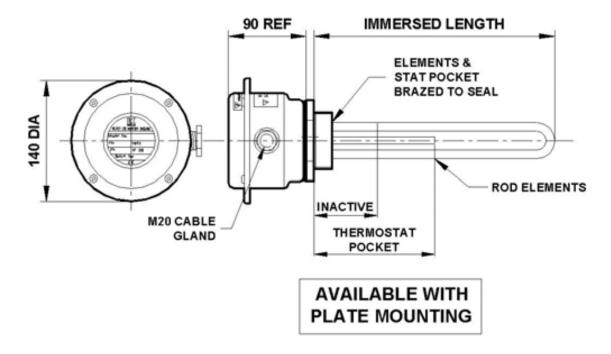
Heat is transferred to the liquid by means of Incoloy 825 sheathed heating elements with automatic control being achieved by the integral adjustable thermostat.
